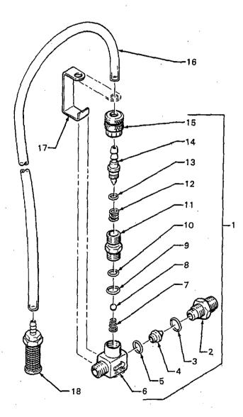
A retaining spring (17) has been installed at the factory to prevent the adjustment knob (15) from being unscrewed too far and the internal parts from falling out. This spring can be removed if the injector needs to be taken apart for cleaning. Be sure to leave spring in place whenever the pressure washer is being used. Removal of spring will not improve chemical flow but could cause chemical injector to quit working.
